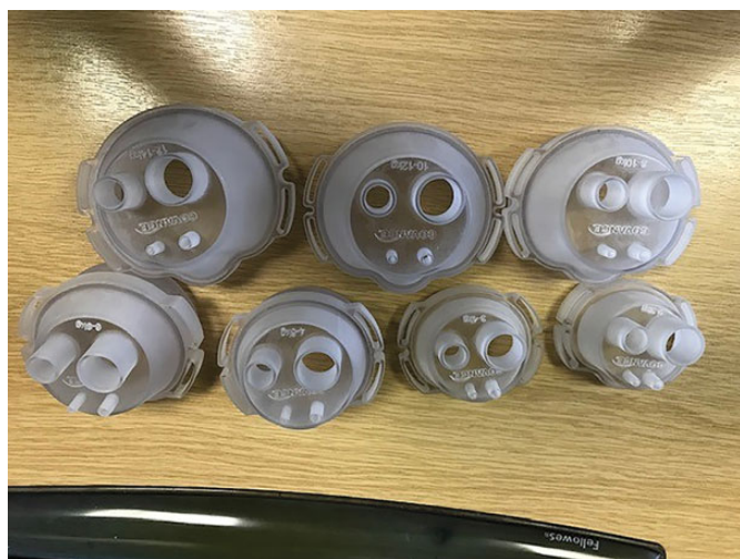
Figure 1. Examples of mature primate masks—Illustration of the variety of face mask sizes required for sexually mature primates on an inhalation toxicity study. Face masks were custom made. Picture courtesy of S. Moore.
